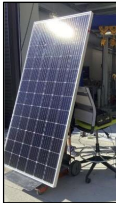
Figure a: Testing of the single panel system under ambient sunlight
